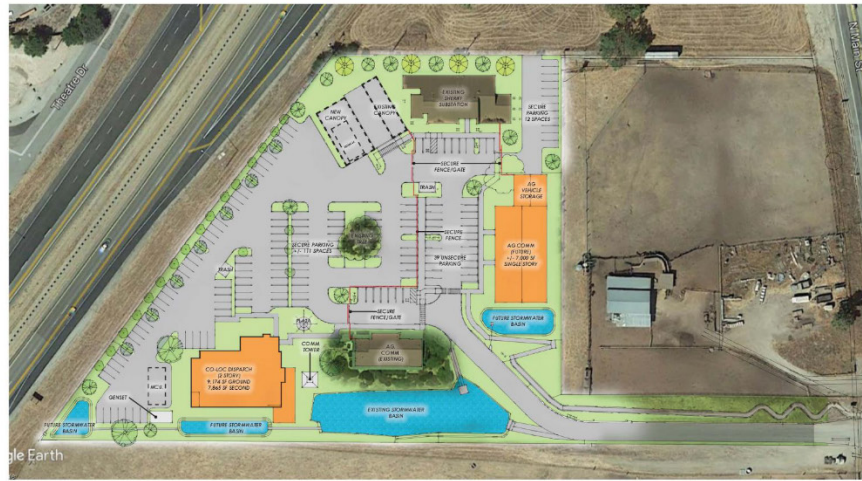
Figure 2. Conceptual Site Plan with Proposed Co-Located Dispatch Facilities and Potential Future Build-Out Facilities
