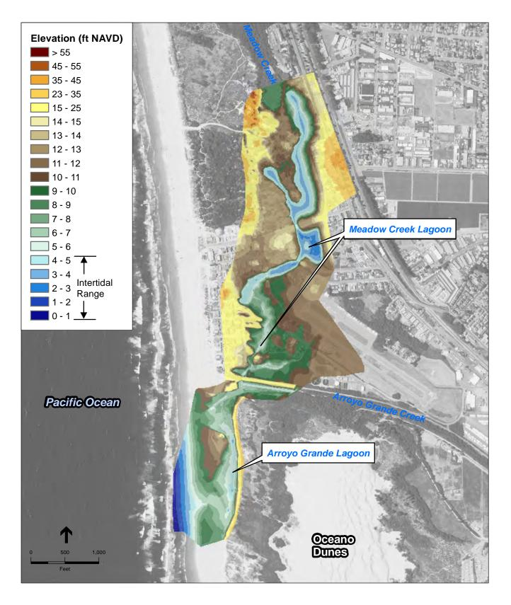
SOURCE: ESA PWA 2011 (survey data), Cannon Engineering 2011 (survey data), NOAA 2010 (LiDAR), NAIP 2012 (air photo) Arroyo Grande Lagoon Interim Sandbar Management Plan . D211720 Figure 8 Topography and Bathymetry
